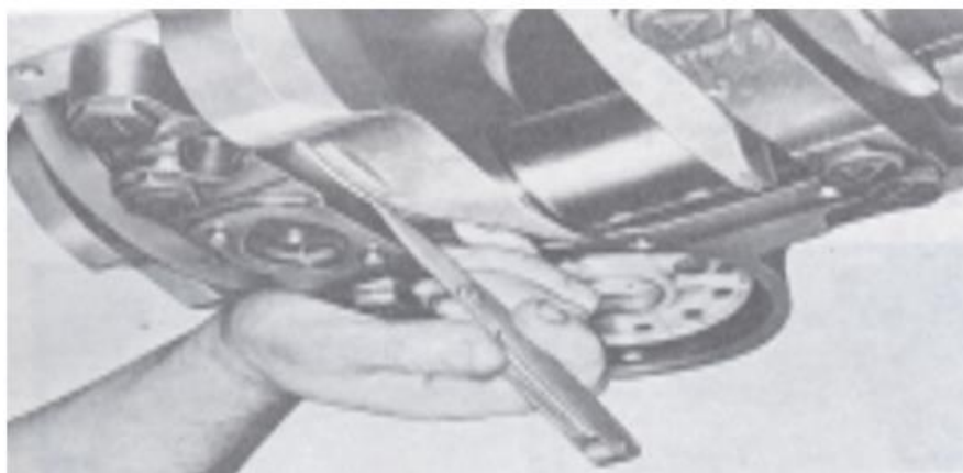
Figure 3. Measurement of axial looseness of crankshaft
