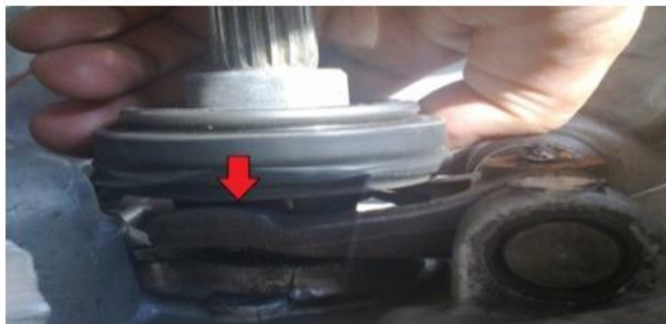
Figure 1. Looseness between bearing nail of clutch and clutch plug
