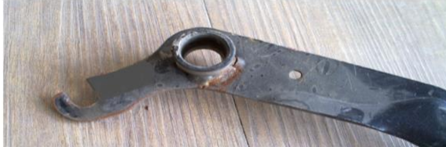
Figure 21. Design of the small arm of non-slotted and non-modified clutch pedal lever
