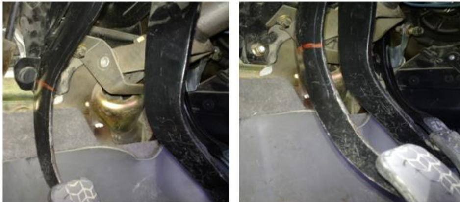
Figure 9. Measurement of length of AD clutch pedal level compared with DE
