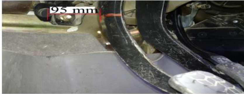
Figure 12. Measurement of DE distance on car
