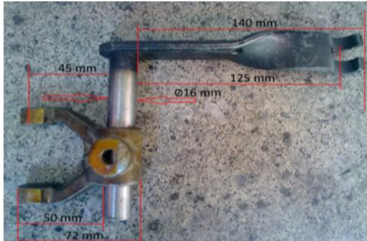
Figure 5. Size of different parts of clutch plug lever
