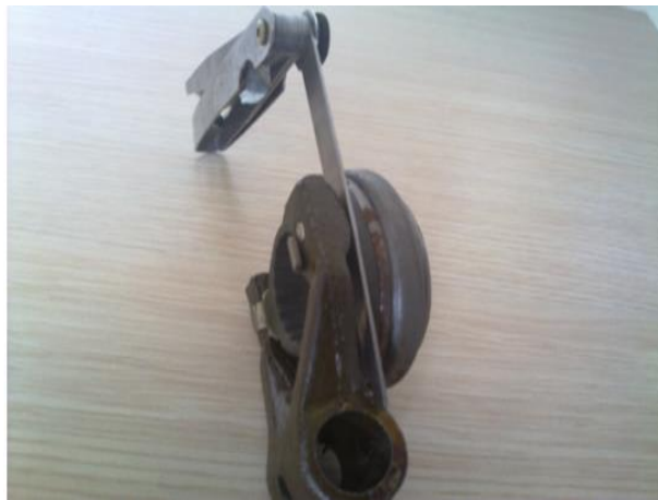
Figure 4. Measurement of distance between bearing nail and clutch plug
