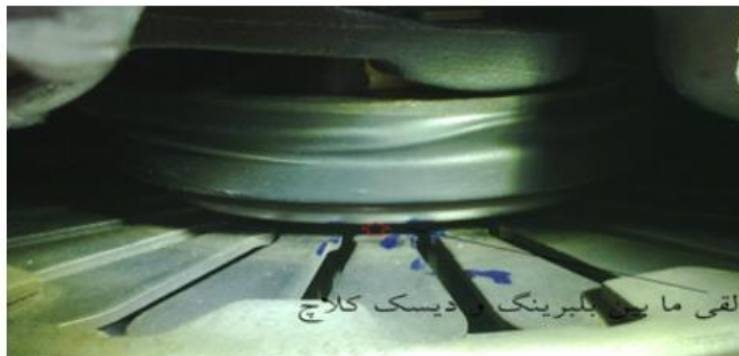
Figure 2. Looseness between clutch bearing and clutch disc
