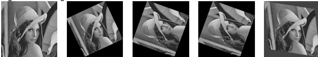
Fig.1.Lena image and attacked versions: (a) un-attacked, (b) rotation 25° (c) rotation70°(d) translation (100,80) and (e) affine transformation[0.9,0.2,0;0.1,1.2,0;0,0,0]
